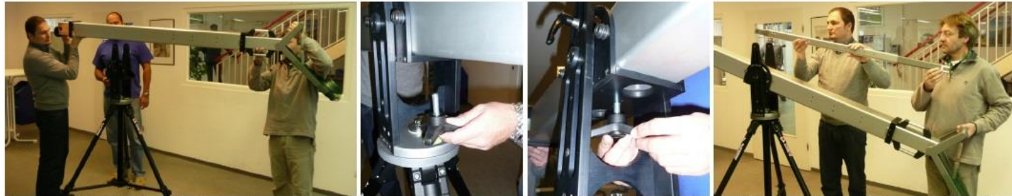
Remove tilt axis from bull stand head and place Movie Jib into it (2 center pins meet 2 holes)
