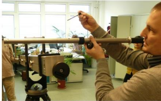
To insert counterweight bar remove quick pin, ...
