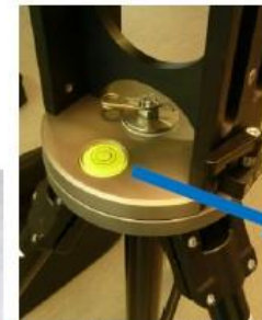
Untighten screw and set the spirit level horizontally
