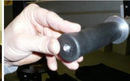
To remove handle push button ...
