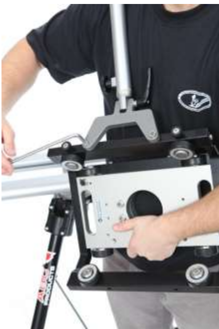
Picture 41 Assembly of the push rod on the dolly frame
