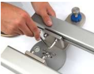
Picture 22 Tighten the slot nut screws with an Allen key
