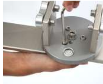
Picture 17 Tighten with an Allen key
