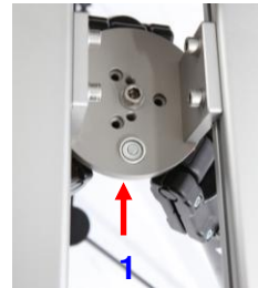
Picture 09 Tracks must be horizontally levelled.
