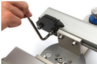
Picture 13 Re-tighten the screws after positioning the end pieces!
