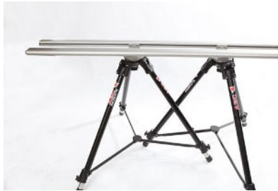
Picture 09 Tracks must be horizontally levelled.
