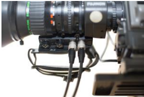
Connector for the focus and zoom function at the lens connecting plate
